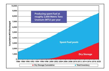
Figure 1.1. US nuclear spent fuel storage; spent fuel pools require electrically powered water pumps to circulate water so heat does not evaporate cooling water. Dry storage does not require electricity. (Source: The Union of Concerned Scientists.)
