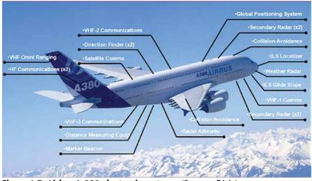
Figure 1.7. Airbus A-380 electronic systems. (Source: FAA.)
